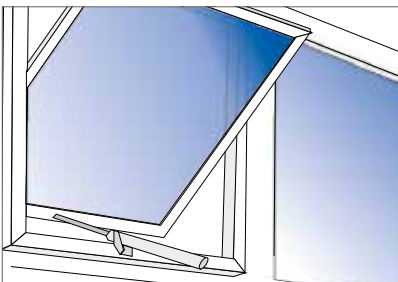
Pivoting window, outward opening at the bottom, with linear drive
