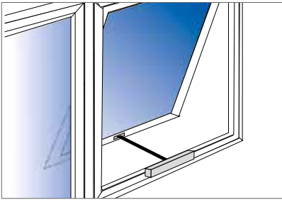
Top-hung window, outward opening at the bottom, with chain drive
