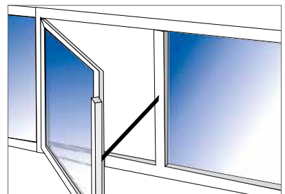
Side-hung window, inward opening, with chain drive
