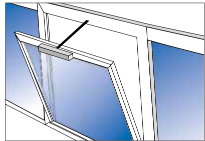
Bottom-hung window, inward opening at the top, with chain drive
